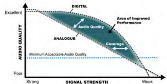
Range and Audio Quality Improvement with DMR Compared to Analog © DMR Association
